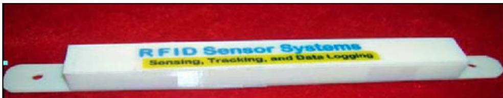
The ST050 passive [EPC](#) Gen 2 tag contains a temperature sensor.
