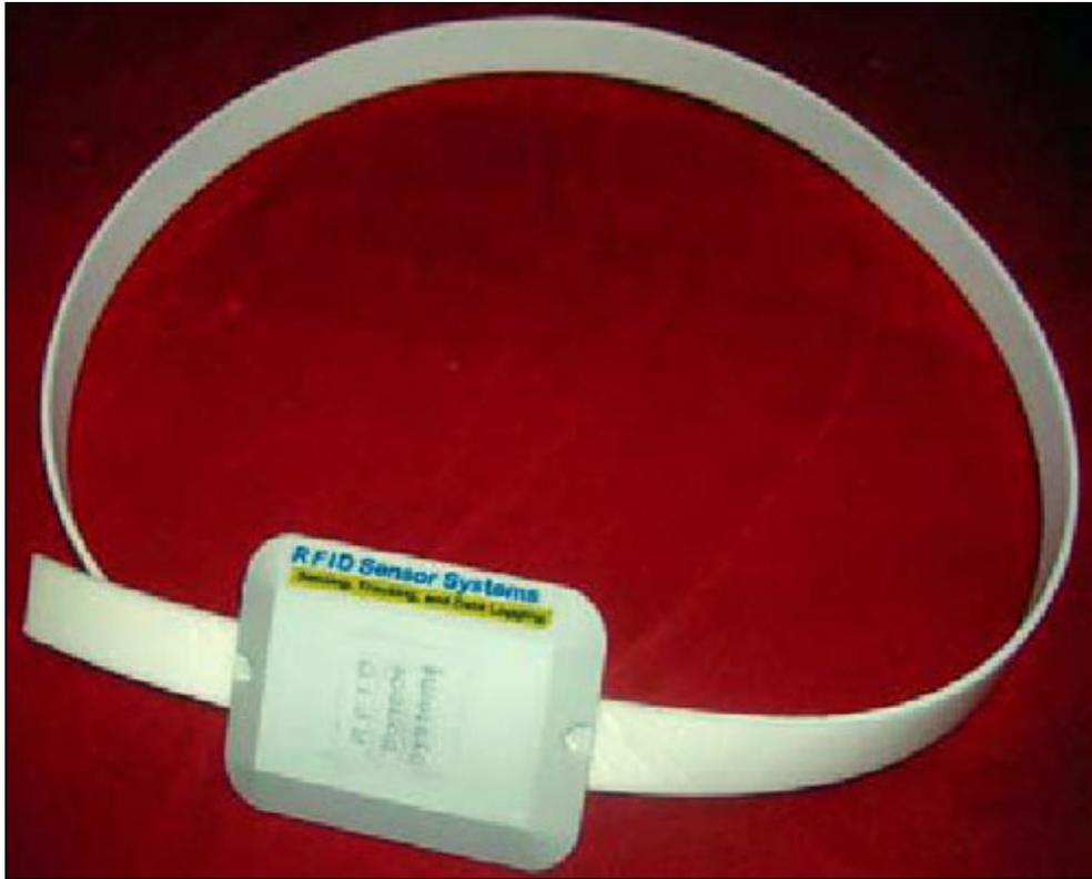
The Cardiopulmonary Monitoring System includes a [tag](#) that can be attached to a patient via a Velcro chest [strap](#) that wraps around the chest.
